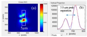
Figure 6: a) Vertically polarized NF image showing two pairs of coherent PSF lobes for two beamlets separated by about 6 µm. b) vertical profile of right hand beamlet with a 5-µm lobe separation which is mapped to 4.6 µm (FWHM) or  $2.0 \mu m (\sigma)$ .
