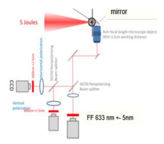
Figure 3: Schematic of the LPA and an early version of the NF and FF imaging setup using the beam splitters to redirect the optical signals to the different cameras [5,6].
