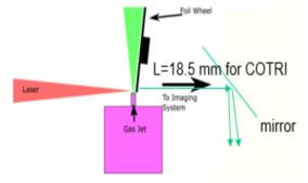
Figure 2: Schematic of the LPA showing the laser, gas jet, and foil geometry at HZDR with a foil separation L= 18.5 mm for COTRI [5,6].
