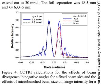
effects of microbunched beam size on fringe intensity for a fixed beam divergence of 0.5 mrad for the positive angles.
