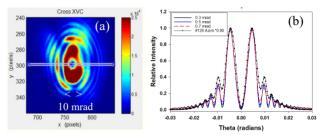
Figure 7: (a) Example of a FF COTRI image at 633±5 nm from the same shot as Fig. 5. (b) Comparison of the azimuthally averaged fringe data and the COTRI model for 0.3,0.5, and 0.7 mrad divergence. The fringe peak positions are well matched, but the relative intensities of some outer fringes are higher in the data. The best match is 0.5 mrad.
