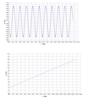
Figure 2: Trajectory of electron along 'x' and 'z in Planar undulator (Numerical calculation).
