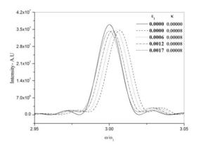
Figure 3: Frequency Spectrum at third harmonics with parameters same given in Table 1,  $\kappa = 8 \times 10^{-5}$  and varying  $\mathcal{E}_1$  from 0 to 17 x 10<sup>-4</sup>.
