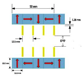
Figure 1: Schematic of one Period of harmonic Undulator(l=3).
