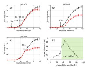
Figure 4: Gain curve comparison between the in- and outphase conditions. One phase shifter is set for the out-phase at (a) 10 m, (b) 30 m, and (c) 50 m. (d) FEL energy difference between the in- and out-phase from the phase shifter scan.
