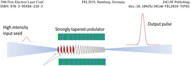
Figure 2: Tapering Enhanced Stimulated Superradiant Amplification - TESSA.
