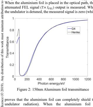
Figure 2: 150nm Aluminum foil transmittance
