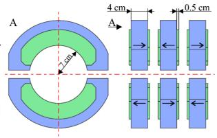
Figure 1: Magnetic design of the undulator. Blue parts are permanent magnets (magnetization is shown with arrows), green parts are iron poles.
