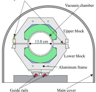
Figure 2: Front view of the undulator.
