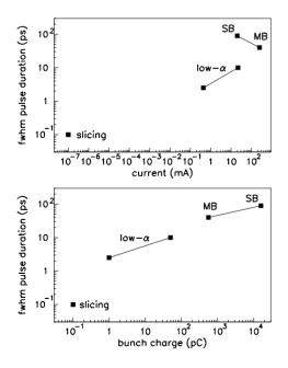
Figure 6: Comparison of femtosecond slicing, low- $\alpha$  operation and normal operation of the BESSY II storage ring with a single bunch (SB) and multiple bunches (MB). Left: pulse duration versus contributing current, which is proportional to the photon flux at the full bunch rate. Right: pulse duration versus contributing change, relevant in the case of pump-probe experiments with a pump pulse rate of 1 kHz.
