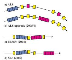
Figure 5: Footprints of femtosecond slicing facilities (not to scale) indicating the respective modulator (blue) and radiator (magenta).
