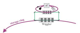
Figure 2: Schematic view of a mm-wave generated by a free-electron laser and interacting with electron bunches in a wiggler, as proposed in [10].
