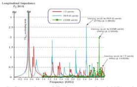
Figure 5: Comparison of  $Z_{\parallel}$  for conventional NC cavity (PEP-II) with HOM-damped NC cavity (BESSY-CS) and SC cavity (CESR-B) [14].
