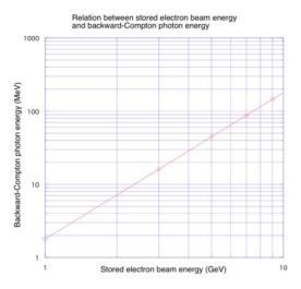
Figure 2: The wavelength  $(10.6\mu m)$  of CO2 laser is fixed and the stored electron beam energy is changed. And a targeted monoenergetic MeV-photon is produced on the axis of just inverse direction against the incident direction of the laser
