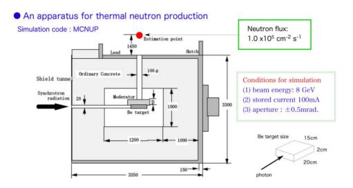
Figure 5: A proposed configuration to obtain thermal neutrons. A block of beryllium target is set up in the center. The most important feature of the method is not to produce radioactive wastes. There is no radiation problem around the apparatus.
