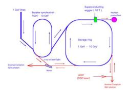
Figure 1: A proposed synchrotron radiation facility consists of a 1GeV-linac, a Booster synchrotron and a Storage ring. A superconducting wiggler with the magnetic field of 10T is installed and supplies MeV-photons to produce neutrons. A collision of CO2 laser and stored electron beam produces MeV-photons through the backward-Compton process. The GeV-photons are also produced with the same process.
