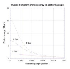
Figure 3: The relation between the energy of inverse Compton photon energy and scattering angle.
