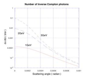
Figure 4: The relation of the cross section and scattering angle.
