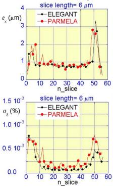
Figure 4: Slice analysis of simulation results trough the BC2 compressor for the horizontal emittance (above), and for the energy spread (below). The 50k particles have been tracked with ELEGANT and PARMELA.
