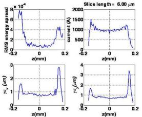
Figure 5: Energy spread, current distribution and transverse emittance along the bunch at the end of the SPARX 1GeV DL1 dogleg, tracked with ELEGANT.
