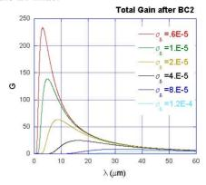
Figure 6: Microbunching gain curve vs. the initial modulation wavelength after the BC2 compressor.
