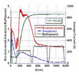
Figure 2: Average current, transverse emittance and envelope, axial magnetic field vs. z for a final 450 A electron beam, tracked with PARMELA [7].
