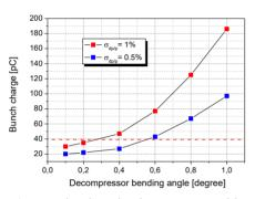
Figure 4: Require bunch charge to provide the peak current of 4kA for different bending angle of the decompressor dipole magnets in the case of different initial RMS energy spread  $\sigma_{\Delta p/p}=1\%$  or 0.5%.
