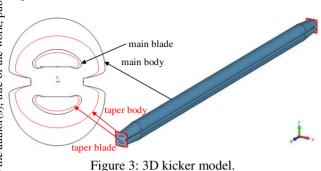
First optimization is extending the vanes to decrease the coupling of the two blades with 3D CST [11]. As shown in Figure 4, the *vane* value changes from *vane* = *b* to *vane* < *b*. The even-mode impedance decreases from ~65  $\Omega$  to <60.5  $\Omega$  as the odd-mode impedance maintains ~50  $\Omega$ . The beam loss factor decreases from 1.042 V/pC to 0.893 V/pC in the Gauss beam ( $\sigma_z = 3$  mm), as shown in Figure 5 that means the beam power loss is about 15% lower.
