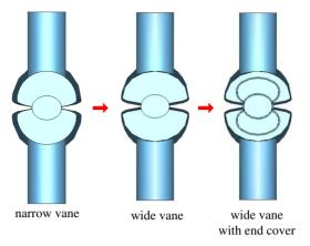
Figure 6: Taper parts improving.
