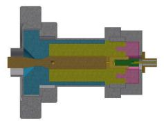
Figure 7: Cross section view of the feedthrough model.
