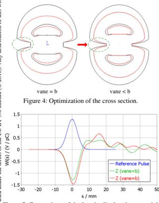
≥ Figure 5: Comparison of the longitudinal wake potential  $rac{1}{r}$  ( $\sigma_z = 3$  mm).
