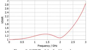
Figure 8: VSWR of the feedthrough.
