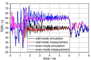
Figure 11: TDR Comparison between simulation and testing results.
