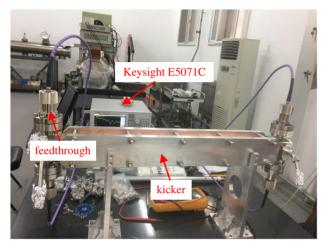
Figure 9: Kicker test setup.
