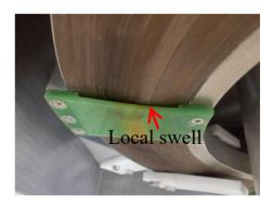
Figure 10: Local damage of type B MA core.
