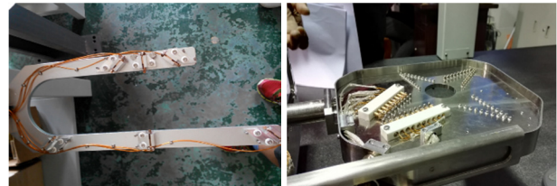
Figure 7: Three wires with 45° angle separating distributed on the frame of the wire scanner, only one wire exposed in the beam pipe at the same time (left); Wires distribution of the multi-wire scanner (right).
