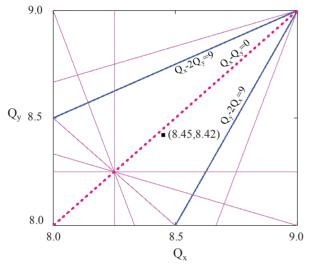
Figure 3: Structure resonances at BRing: 3<sup>rd</sup> order (blue solid), 4<sup>th</sup> order (pink solid); linear coupling (red dash).
