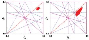
Figure 5: Tune spread of coasting (left) and bunched (right)  $U^{34+}$  beam after filling up the transverse acceptance. The dot " $\blacksquare$ " marks the nominal working point at the BRing.
