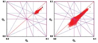
Figure 6: Tune spread of coasting (left) and bunched (right)  $U^{34+}$  beam with emittances of 50/50  $\pi$ mmmrad.
