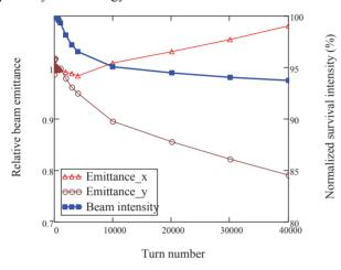
Figure 7: Simulation of relative emittance at horizontal (red " $\Delta$ ") and vertical (brown " $\circ$ ") planes after filling up the transverse acceptance, and normalized survival beam intensity (blue " $\blacksquare$ ") during RF capture process from initial coasting beam.
