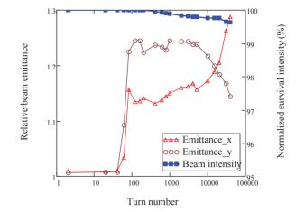
Figure 8: Simulation of relative emittance at horizontal (red " $\Delta$ ") and vertical (brown " $\circ$ ") planes with 50/50  $\pi$ mmmrad emittance, and normalized survival beam intensity (blue " $\blacksquare$ ") during RF cavity capture process from initial coasting beam to bunch.
