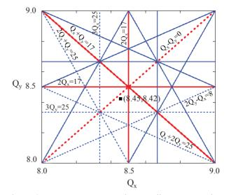
Figure 4: Betatron resonances in tune diagram at BRing: 2<sup>nd</sup> order (red solid line), 3<sup>rd</sup> order (blue solid line); resonance stop-bands to be compensated (dash line). The nominal working point (" $\blacksquare$ ") for <sup>238</sup>U<sup>34+</sup> operation is set as (8.45, 8.42) at injection energy.
