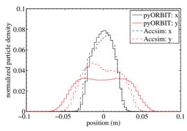
Figure 11: Projections onto the horizontal axis (black) and the vertical axis (red), working point *c*. A comparison between pyORBIT (solid line) and Accsim (dashed line).
