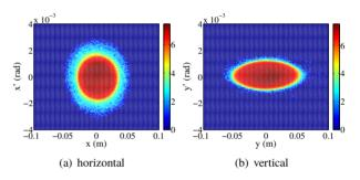
Figure 9: Density plots of the horizontal (a) and vertical (b) phase space. The colorbar marks the density in log scale.
