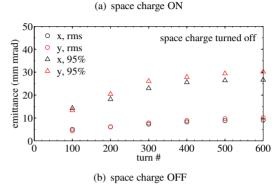
Figure 12: Emittance evolution during injection obtained with Accsim when space charge is turned on (a) and off (b) in the simulation.
