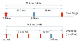
Figure 2: Sketch of the different accumulation scenarios. Protons pulses are in blue and H<sup>-</sup> pulses are in red.
