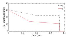
Figure 5: The closed orbit bump (c.o.) amplitude as a function of time. At the end of the injection, at  $t=0.73\,\mathrm{ms}$  corresponding to 550 injected turns, the bump amplitude is set to zero for computational ease. In reality it takes some microseconds to completely remove the bump.
