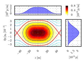
(a) Double-harmonic bucket in BLM (i.e. 180° relative phase and  $V_{h=2} = V_{h=1}/2$  populated with a matched distribution (note the quasi-Gaussian distribution in the momentum projection).
