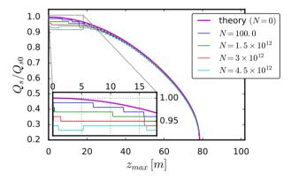
Figure 4: Normalised actual synchrotron frequency  $Q_S/Q_{S,0} \equiv \omega_S/\omega_{S,0}$  vs. synchrotron amplitude expressed in  $z_{\text{max}} = \tilde{\phi}R/h$ , the violet line corresponds to Eq. (6).
