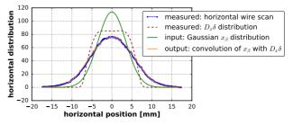
Figure 6: Wire scan comprising betatron and dispersive part.
