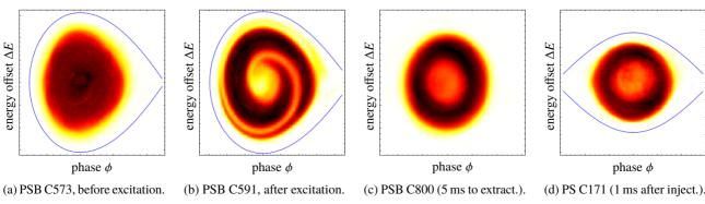
Figure 5: Longitudinal phase space ( $\phi, \Delta E$ ) reconstructed via tomography at different stages in the PSB (measurements) [5].
