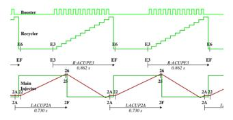
Figure 2: Relative timing of Booster, Recycler and Main Injector cycles for NO $\nu$ A-era NuMI operation. Beam in each machine is shown in green, and Main Injector momentum in red. The start and end of cycle clock events for MI and Recycler are also shown.
