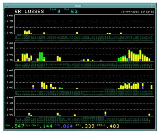
Figure 5: Loss around Recycler for 525 kW operation April 2016.
