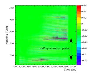
Figure 7: The fast recycler instability in the horizontal plane. The color scale represents horizontal motion, in arbitrary units. Shown is the first injected batch  $(1.6 \,\mu\text{s})$  for about 500 turns after injection. The incoming beam is not perfectly matched to the rf bucket here, and the instability is seen to occur at bunch length minima, and in the center and the end of the batch.
