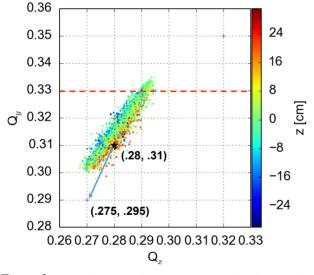
Figure 3: Tune footprint of the beam in LHC with octupoles powered to -20 A, chromaticities  $Q'_{x,y}$  set to 15/20, and assuming an EC density of  $5 \times 10^{11}$  e/m<sup>3</sup> uniformly distributed along the whole ring.
