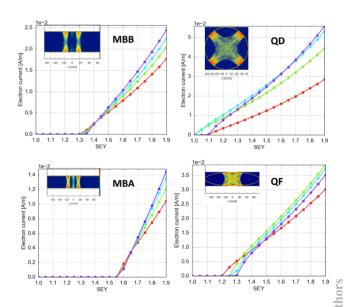
Figure 2: SEY curves for EC formation in the four types of SPS chambers (dipoles on the left and quadrupoles on the right side) and for four different bunch intensities (red  $1.0 \times 10^{11}$  p/b, green  $1.5 \times 10^{11}$  p/b, turquoise  $2.0 \times 10^{11}$  p/b, purple  $2.5 \times 10^{11}$  p/b).
