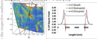
Figure 9: Ring Tune plane scan (left) and Main ring dipole multipole field distributions from OPERA model
