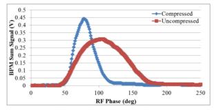
Figure 10: Position monitor line density vs RF phase for compression (blue) and normal operation (red).
