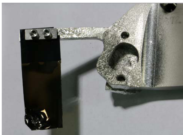
Figure 5: An SNS stripper foil bracket showing damage due to reflected convoy electrons. Photo by Chris Luck.
