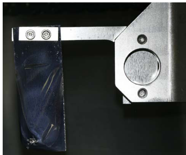
Figure 6: A TZM bracket used at 1.3 to 1.4 MW for about 16 days. Photograph by Chris Luck.
