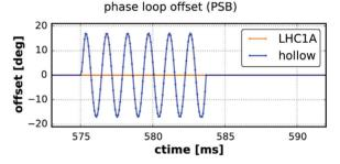
Figure 4: Trim function for the phase loop offset (blue curve).
