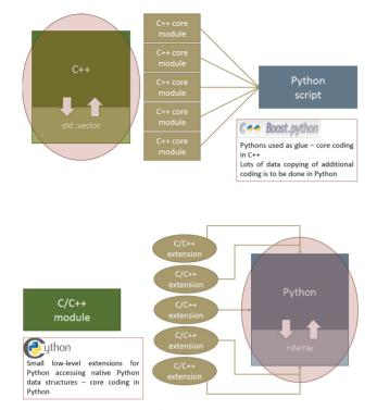
Figure 3: Comparison of the two strategies using Python as a "glue" language (top) and using Python as the core programming language (bottom) with the lower level language being C++ in this example. The core programming language is encircled in red in each case along with the basic data structure used.
