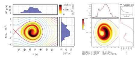
Figure 5: Comparison of the longitudinal phase spaces as obtained in simulation and measured in the experiments. Note that the horizontal axis on the left plot indicated position whereas on the right plot it indicates time.
