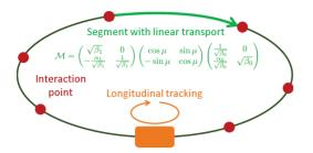
Figure 1: Illustration of the typical numerical model of the accelerator-beam system for collective effects.  $\alpha$ ,  $\beta$  denote the Twiss parameters,  $\mu$  the phase advance between the interaction points (red).
