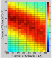
Figure 3: Transmission rate of the CPHS RFQ with the currents of the two solenoids.
