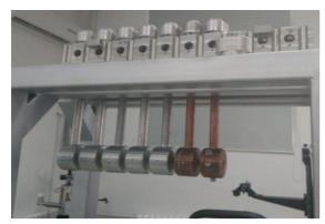
Figure 5: Alignment experiment with the test drift tubes.
