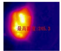
Figure 4: Temperature distribution of the Be target with the proton beam bombarding on it.
