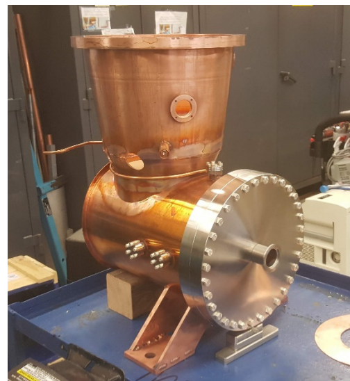
Figure 13 : The partially assembled cavity.
