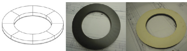
Figure 3: Layout and photographs of the garnet and alumina sides of a tuner ring.
