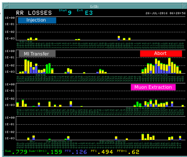
Figure 5: Typical loss pattern around the Recycler before the 2016 summer shutdown. Intensity is 42E12 ppp.
