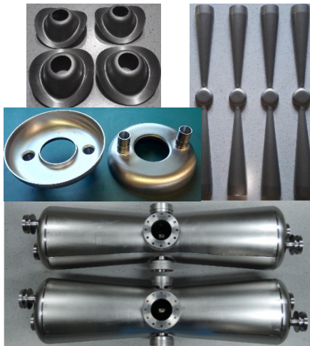
Figure 7: Fabrication of \beta_g=0.09 HWR cavity.
