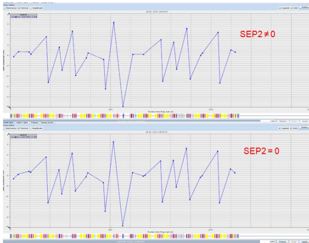
Figure 3: Vertical circular beam orbits while the power of the septum-2 magnet is on (above) or off (below).
