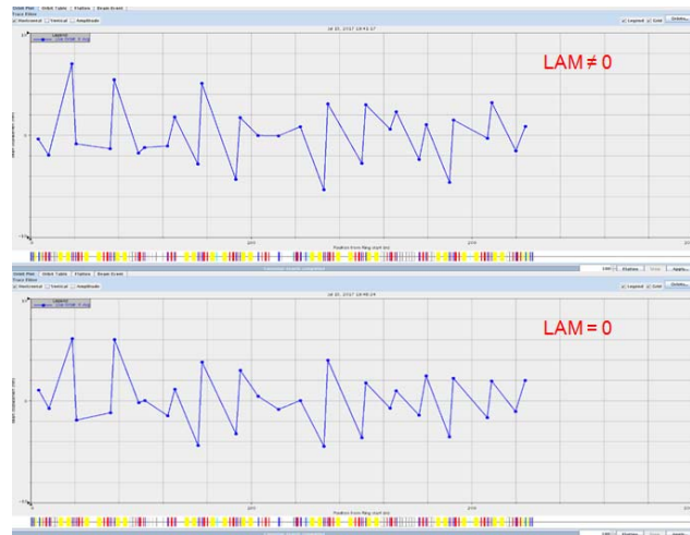
Figure 4: Horizontal circular beam orbits while the power of the lambertson magnet is on (above) or off (below).
