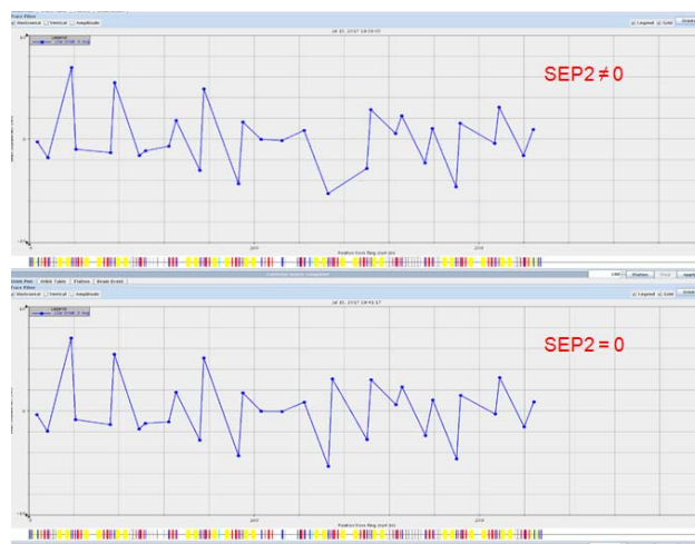
Figure 2: Horizontal circular beam orbits while the power of the septum-2 magnet is on (above) or off (below).
