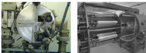
Figure 15: Film irradiation device of IC100 [4] (left) and DC110 [8] (right) cyclotrons.
