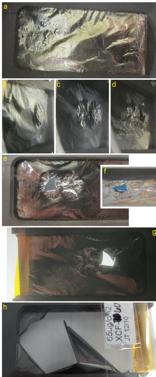
Figure 4: a) Foil before irradiation. b-d) After 1 st /2 nd /3 rd fraction, in vacuum. e-g) Afterwards in air. h) Other foil, damaged at mounting. a,e,f,h) front, b-d, g) rear side.
