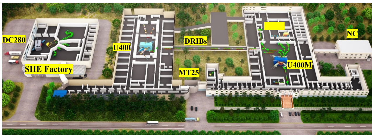
Figure 1: The layout of the Flerov Laboratory buildings, where: U400, U400M, IC100, DC280 are heavy ion cyclotrons, MT25 is microtron, SHE Factory is Super Heavy Element Factory, NC is Nanotechnology Centre.
