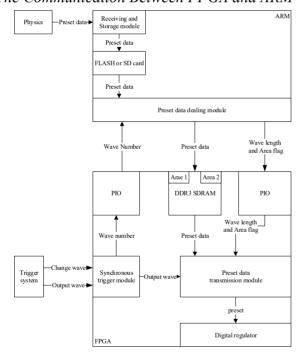
Figure 2: Pre-set data transmission flow.
