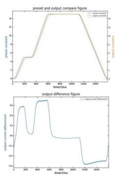
Figure 7: The pulse given and output current (the above one) and the error between given and output (the bottom one).
