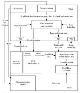
Figure 3: Read-back data transmission flow.
