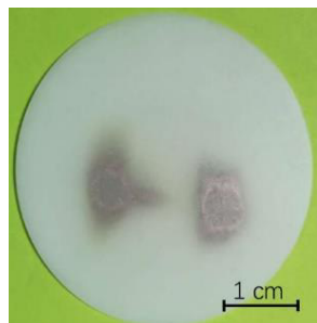
Figure 4: The ^{63}\text{Cu} and ^{65}\text{Cu} spots on the secondary target from right to left.
