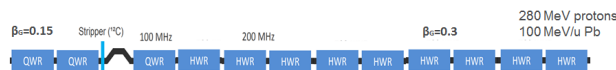
Figure 7: Schematic layout of the SRF section of the JLEIC including a stripper section after the second QWR module.
