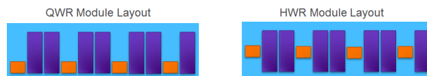
Figure 8: Layouts of the QWR and HWR cryomodules each with seven cavities and four solenoids.
