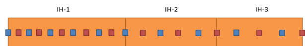
Figure 6: Layout of the DTL section made of 3 tanks including 19 accelerating gaps and 20 quadrupoles in a FODO lattice arrangement.
