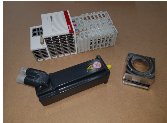
Figure 14: The stepper motor and associated controller units have arrived at NTG and will be integrated into ROSE to replace the GSI systems.
