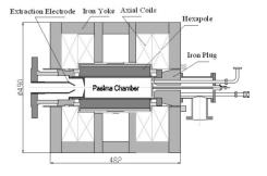
Figure 7: Schematic drawing LECR3 source.
