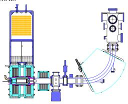
Figure 8: LECR4 source test bench layout.
