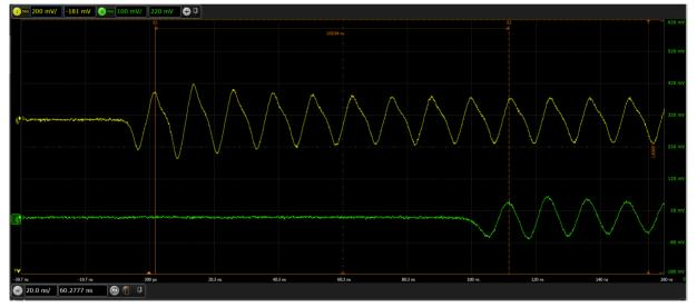
Figure 5: Measured signals of N<sup>2+</sup> beam current from two BPMs.
