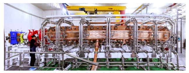
Figure 2: Side view of installed RFQ after full assembly on site.
