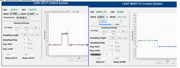
Figure 4: Measured signals of N<sup>2+</sup> beam current form ACCTs and a Faraday Cup.
