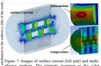
Figure 7: Images of surface current (left part) and multiphysics analysis. The intensity increases as the color changes from blue to yellow and to red.
