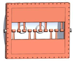
Figure 3: The inner structure of proposed HOM-DTL.
