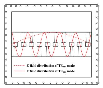
Figure 4: RF property of TE<sub>115</sub> mode (solid line) in the HOM-DTL. Dot line shows RF property in IH-DTLs.
