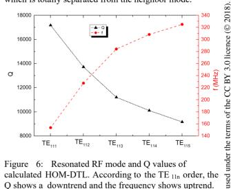
Figure 6: Resonated RF mode and Q values of calculated HOM-DTL. According to the TE 11n order, the Q shows a downtrend and the frequency shows uptrend.
