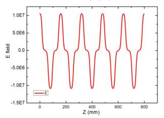
Figure 5: Flat e field distribution of TE<sub>115</sub> mode in the HOM-DTL.
