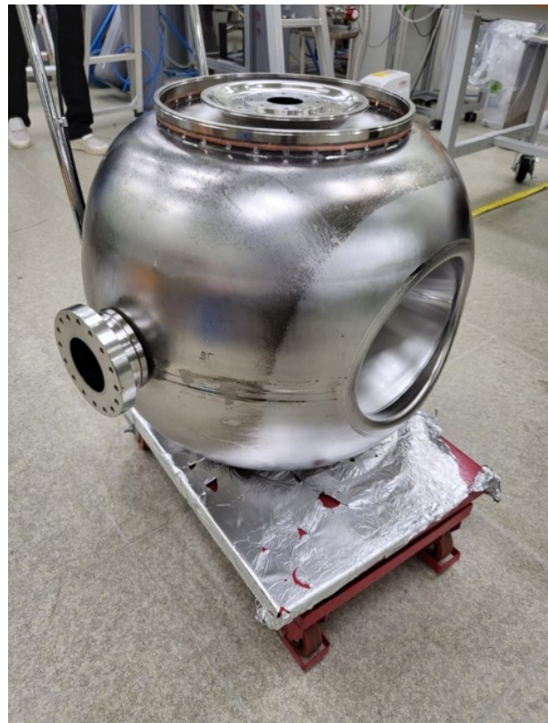
Figure 2: Fabricated SSR2 Bare Cavity.
