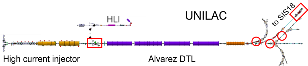
Figure 1: The UNILAC and its main constituents: The high current injector with two source terminals and an RFQ/IH-DT linac (left), the high charge state injector HLI (top centre), and the main Alvarez-DT linac (centre). To the right are several user branches and the transfer channel to the synchrotron. Stripper sections for general accelerator operation are framed with red boxes, strippers for special user requirements with red circles.
