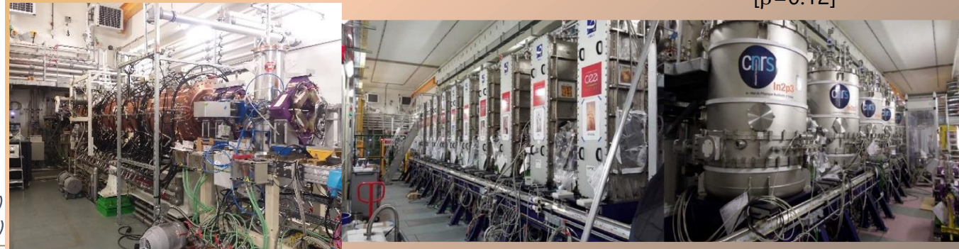
RFQ 88 MHz Superconducting cryomodule A [ \beta=0.07 ] Superconducting cryomodule B [ \beta=0.12 ]
