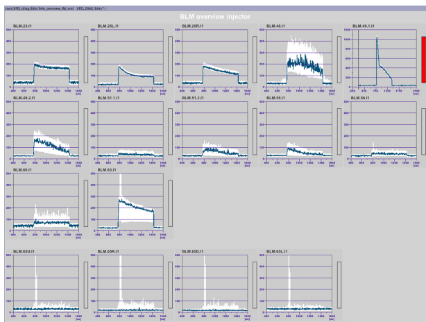
Figure 4: Display of the beam loss monitors during beam operation. Most of the monitors show the continuous dark current background, one BLM.49 produces an alarm (indicated in red). The BLMs in the dump line (bottom row) show in white color history data from previous trains.
