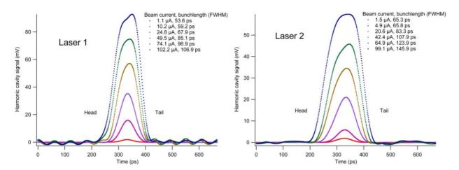
Figure 3: Bunchlength measurements made with the harmonically-resonant cavity of 499 MHz electron beams using "laser 1" with 45 ps optical pulsewidth FWHM (top), and 249.5 MHz beams using "laser 2" with 60 ps optical pulsewidth FWHM (bottom), for different extracted beam currents. These plots were obtained by transforming the raw oscilloscope waveforms using an estimate of the harmonic cavities transfer function.
