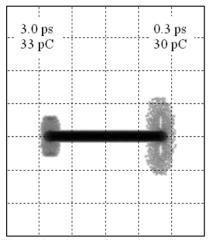
Figure 6: The probe electron beam images on the observation screen for 3.0 (left) and 0.3 ps (right) long bunch, bunch charges are 33 and 30 pC respectively (low alpha BESSY VSR mode); grid size is 2 mm.
