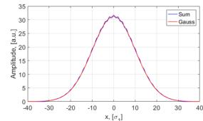
Figure 3: Representation of the long Gauss as a sum of the short ones – the blue curve, see Eq. (2), and Gaussian distribution – the red curve.
