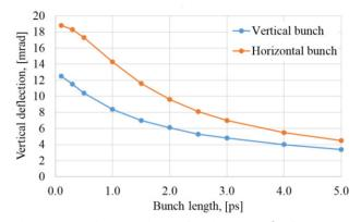
Figure 4: Maximal vertical deflection angle  $\theta_y$  of the probe electrons as a function of the bunch length for vertical and horizontal bunch orientations.
