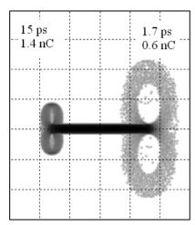
Figure 5: The probe electron beam images on the observation screen for 15 (left) and 1.7 ps (right) long bunch, bunch charges are 1.4 and 0.6 nC respectively (standard BESSY VSR mode); grid size is 2 mm.
