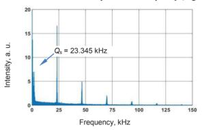
Figure 5: Synchrotron frequency obtained by Fourier transform of the dissector signal.
