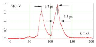
Figure 8: The two laser pulses separated by a 10-ps time interval acquired by the dissector.
