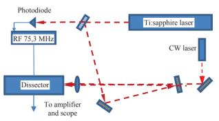
Figure 6: The scheme of the experiment for direct measurement of the temporal resolution of the dissector.
