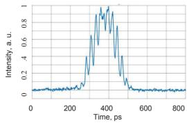
Figure 4: Distortions of the signal of the dissector caused by synchrotron oscillations.
