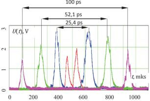
Figure 7: Pairs of the laser pulses acquired by the dissector at different time intervals between them.
