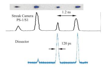
Figure 9: The longitudinal bunches profiles acquired by streak camera PS-1/S1 and the dissector
