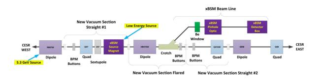
Figure 2: NGXBSM functional diagram.
