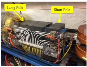
Figure 4: NGXBSM source magnet.
