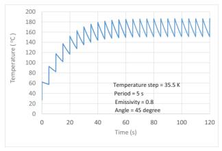
Figure 5: Simulations of steady state temperature.
