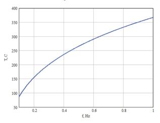
Figure 4: Steady state temperature of YAG crystal depending on e-beam repetition rate.
