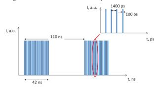
Figure 2: Temporal structure of electron beam.
