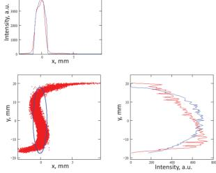
Figure 3: Typical beam profile on YAG screen (red) and equivalent ellipse (blue) homogeneously filled with the same number of particles. For the ellipse, only the outline is shown on the plot.
