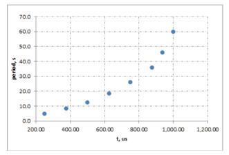
Figure 6: Period between bunch trains depending on train length. For each case YAG steady state temperature does not exceed 186 C.
