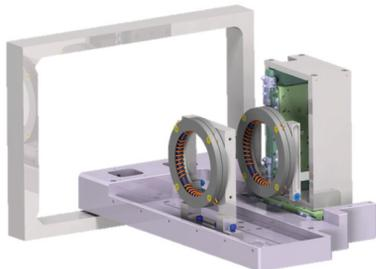
Figure 2: Schematics of the measurement setup, which was installed in the accelerator COSY. Front Rogowski coil BPM is mounted to a fixed frame. The rear one is mounted on a piezo table, which can be moved in horizontal and vertical direction.
