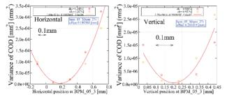
Figure 5: Beam-based alignment data from one of the BPMs. Left and right plots show horizontal and vertical directions, respectively.
