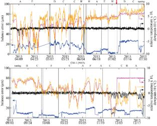
Figure 4: Trend graphs of the balance error of a current BPM (blue lines). The upper figure shows the data before the cable replacement and the lower one is those with new cables. The dew point of the accelerator tunnel (electronics area) is plotted by a magenta (orange) lines. The relative electronics temperature (x10) is shown by black lines.
