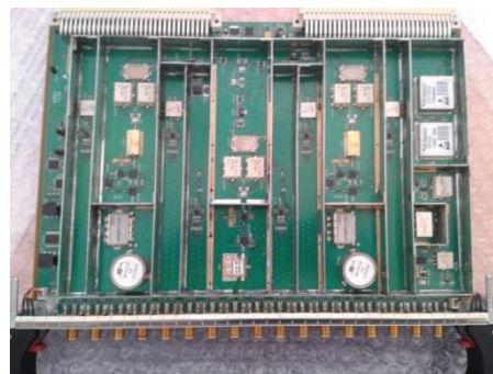
Figure 1: Reentrant RFFE board.
