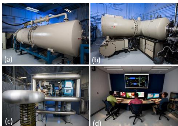
Figure 2: MIBL particle accelerators: (a) 3 MV Tandem – Wolverine (W), (b) 1.7 MV Tandatron – Maize (M), (c) 400 kV ion implanter – Blue (B) and (d) view of the Control Room (CR) of the three accelerators that now operate in remote control mode.
